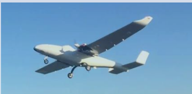
180kg, >10h, 500km(SATCOM) EO/IR, Mar. radar, Still camera, radar detector, phone detector, EPIRB
