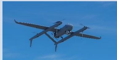
47.6kg, >9h, 140km EO/IR with automatic scanning mode, EPIRB VTOL (incl. from vessels)
