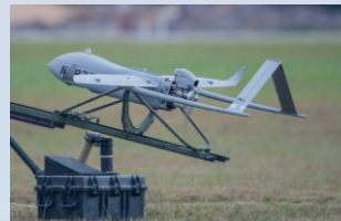
36kg, >10h, 140km, up to 400km with ground relays EO/IR, radar Launcher & net
