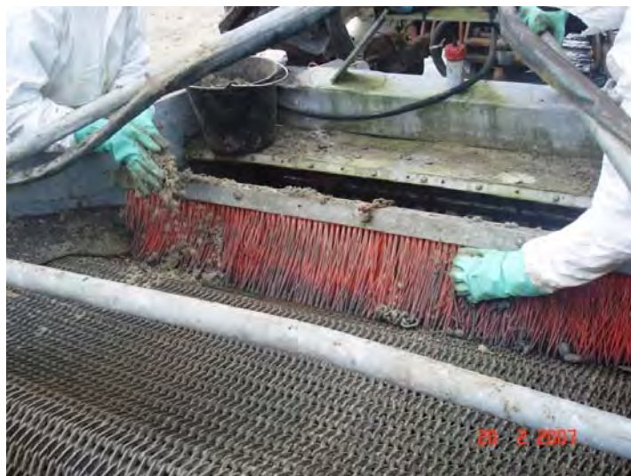
Mechanical sand/gravel/pebble sieving (Source: Le Floch Depollution)
