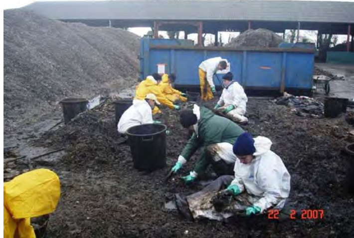
Sorting of waste prior to pre-treatment (required in the absence of sorting during collection) (Source: Le Floch Depollution)
