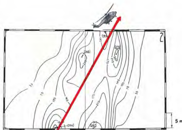
The litres per hectare iso-spraying curve for a SOKAF Bucket dispersant spraying system (mesh size of the map is 5 metres for a spraying rate in litres per hectare)
