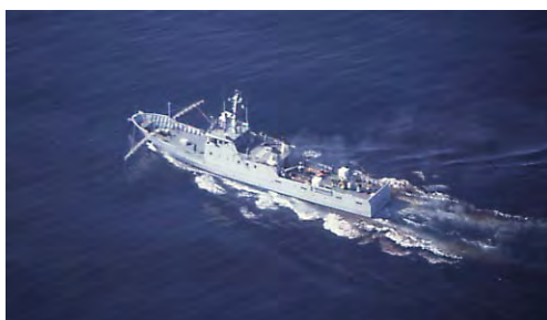
Figure 8: Ship applying dispersant (a part of mixing energy is generated by the bow wave)
