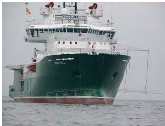
Figure 20: Ship mounted modern application spraying equipment (source SINTEF)
