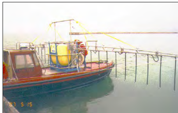
Figure 27: Conventional dispersant spraying system for boat
