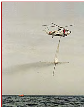
Figure 26: Helicopter equipped with independent spraying bucket (source SINTEF)
