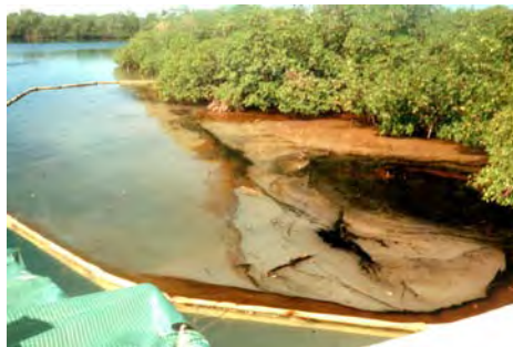
Figure 14: Field experiment conducted on mangrove with dispersed oil in order to assess the impact of the dispersion in TROPIC experiment (source: Clean Caribbean)
