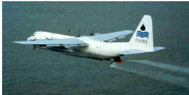
Figure 24: Large Self Contained spraying system (20t capacity) on C130 Hercules
