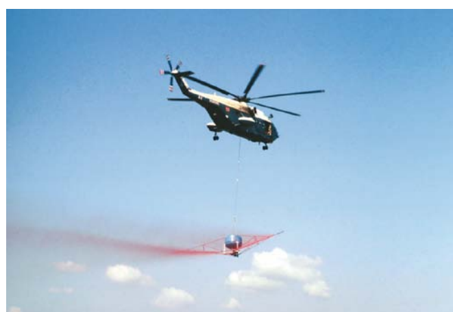
Dispersant spraying modes for vessels, planes and helicopters.
