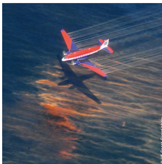
Figure 22: Spraying multi-engine aircraft during Deep Water Incident (source US Coast Guard)
