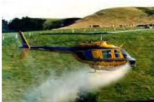
Figure 25: Fixed spraying systems for helicopter
