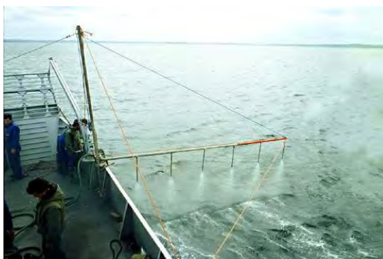
Figure 28: Application of dispersant pre-diluted into sea water
