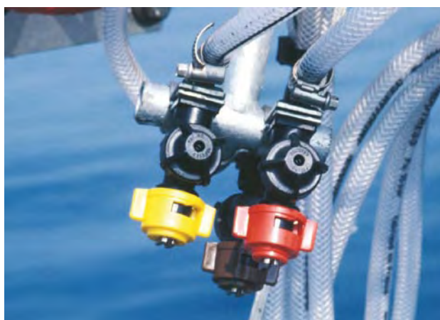
Nozzles fitted with check valves.
