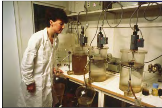
Figure 16: The IFP / flow through test apparatus (source SINTEF)
