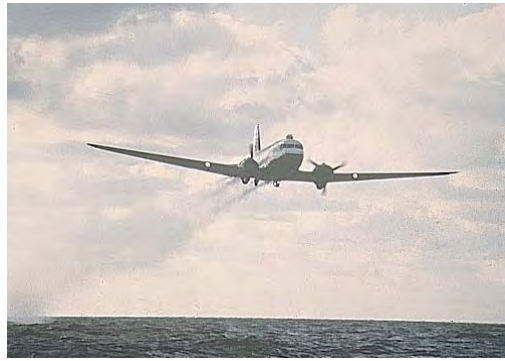
Figure 5: Aerial dispersant application with a DC3 aircraft from the UK authorities (source MPCU)
