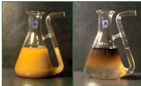
Figure 17: The swirling flask test method (source: www.marinemangement.org.uk/protecting/pollution/documents/approval_lr448.pdf )
