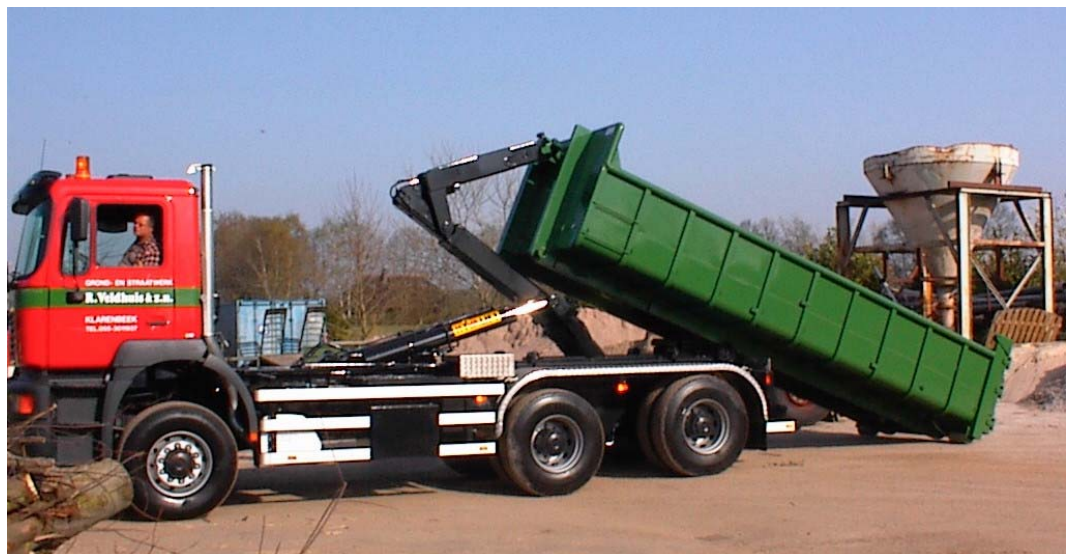
Figure 7.4: Hook lift system
