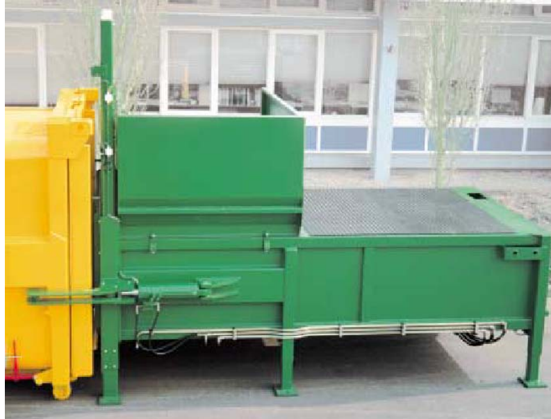
Figure 7.5: Stationary press connected to a press container
