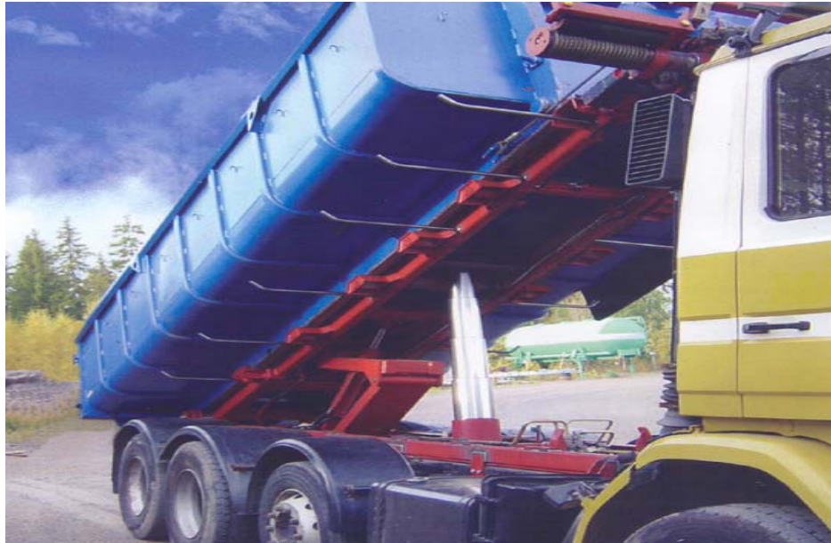
Figure 7.3: Cable lift system
