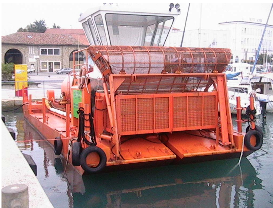
Specialized spilled oil and garbage collection vessel operated by the Harbour Master local office
