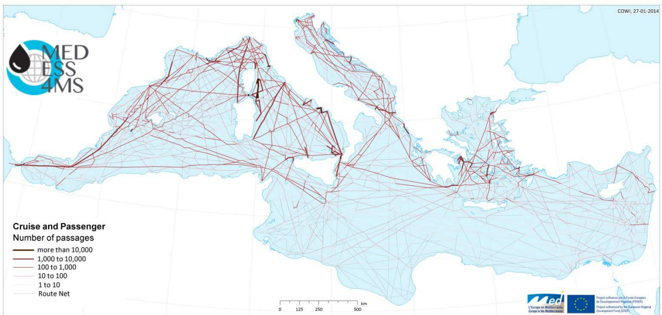
Figure 5-4 Map of the total traffic intensity on route segments of cruise and passenger vessels larger than 300 GT in period 1 February 2013 – 31 July 2013.
