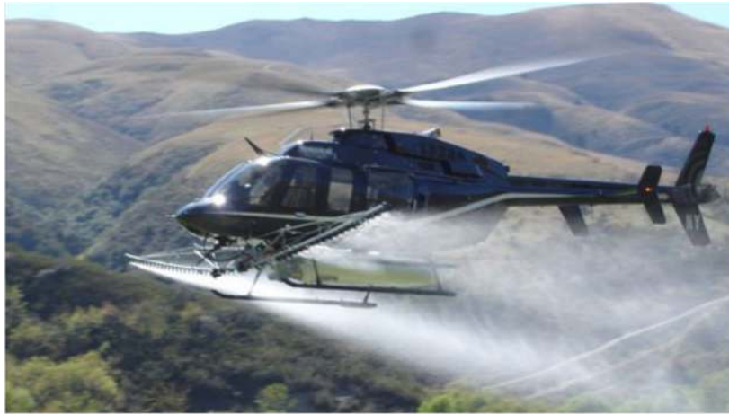
Figure 24. Fixed spraying systems for helicopter (©Dart Aerospace)
