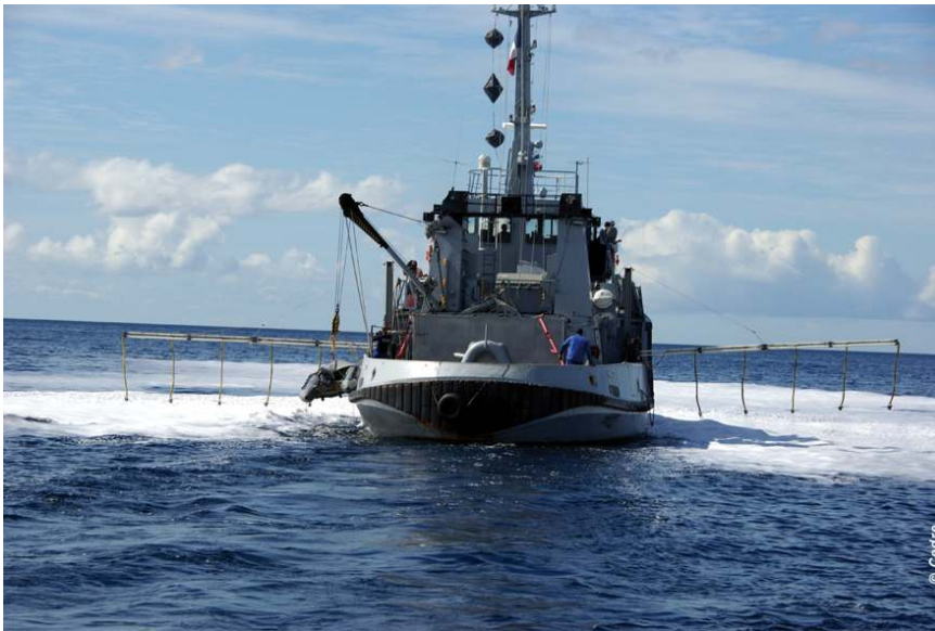
Figure 13. Spraying dispersant by boat during a POLMAR exercise in Saint-Barthelemy (France) (©Cedre).
