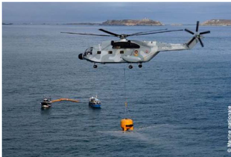
Figure 25. Dispersant bucket used during a Polmar-Terre/Mer exercise in Côtes d'Armor (France) (© French Navy)
