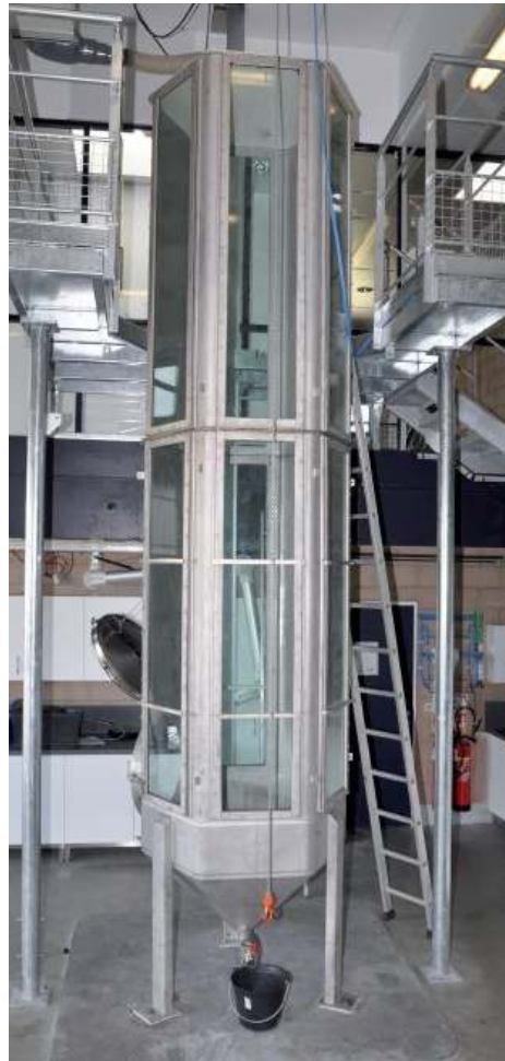
Figure 12. Cedre's experimentation column (©Cedre). Objective : visualize the formation and stability of dispersed hydrocarbon droplets in the water column.
