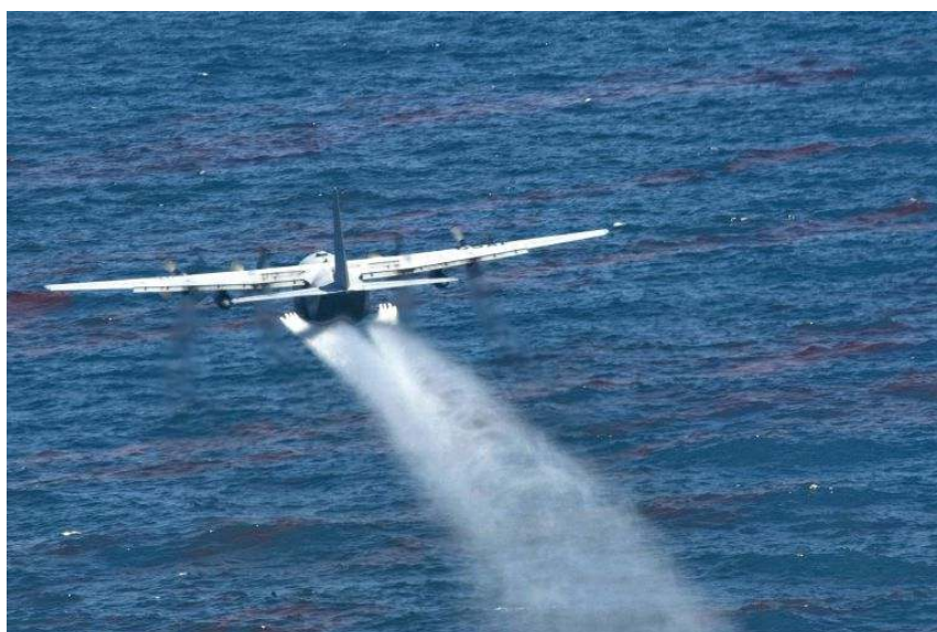
Figure 5. A U.S. Air Force chemical dispersing C-130 aircraft as part of the Deepwater Horizon Response on the surface (© US Coast Guard photo)
