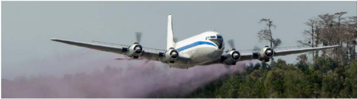
Figure 18. Example of fixed systems on aircraft wing. Florida Air Transport DC-6 (N70BF) performing spray tests (Source: http://floridaairtransport.com/index.php ).
