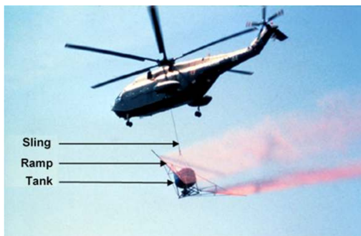
Figure 23. French Navy Super Frelon heavy-lift helicopter fitted with bucket system (© Cedre).
