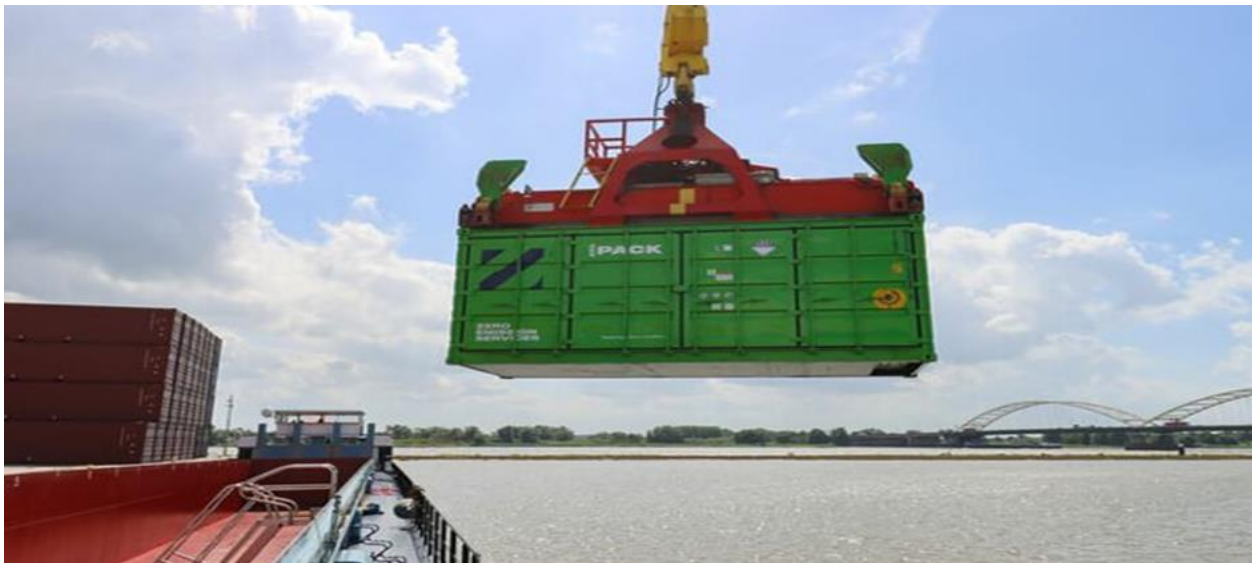
Figure 3.7 Swappable batteries pack
