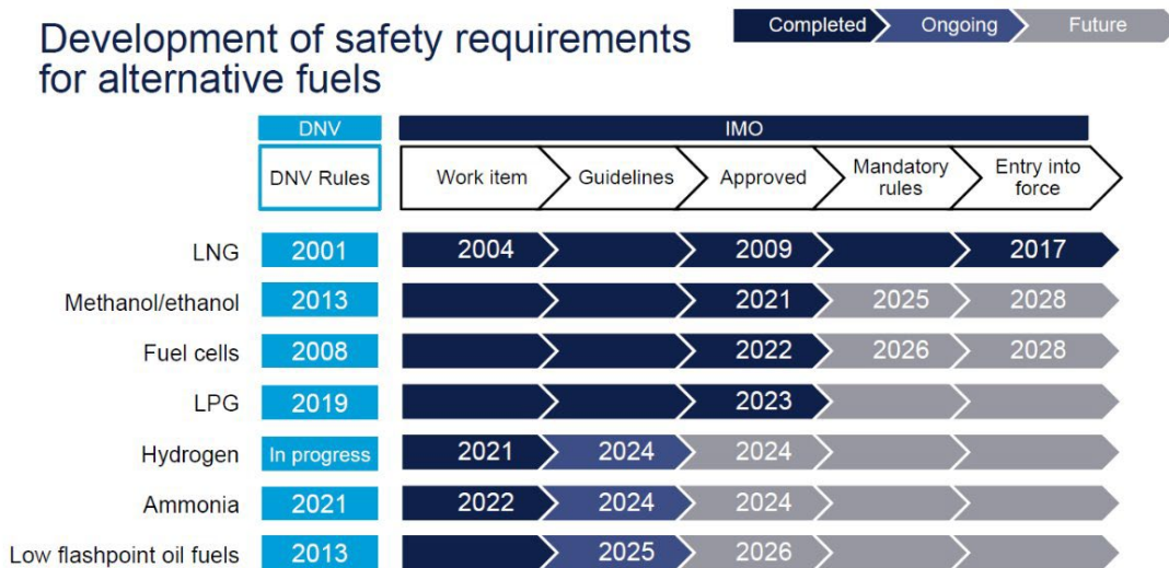
Figure 4-3: Development of safety requirements for alternative fuels. Source: Updated work plan for the development of new alternative fuels under the International Code of Safety for Ships using Gases or other Low-flashpoint Fuels (IGF code), CCC 9/WP.3, Annex 3, various IMO documents and DNV estimates. Future dates are indicative.
