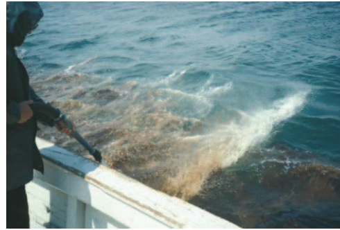
1., 2. Dispersion trial. See the beige colour of the slick just after spraying. This effect will last once a fire monitor has jetted the oil and dispersant.
