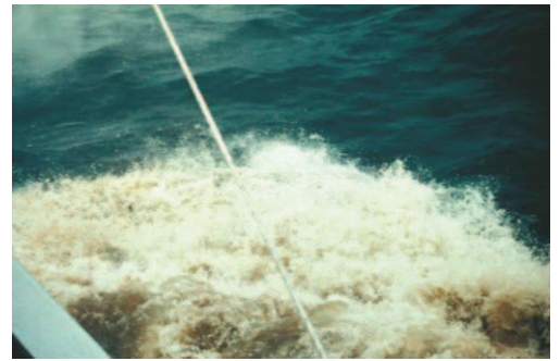
3. Effect caused by the bow wave of a vessel passing through a treated slick. See the beige colour in the foam.
