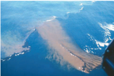
4. When the wave goes through the treated slick, oil is placed in suspension and the beige cloud forms.
