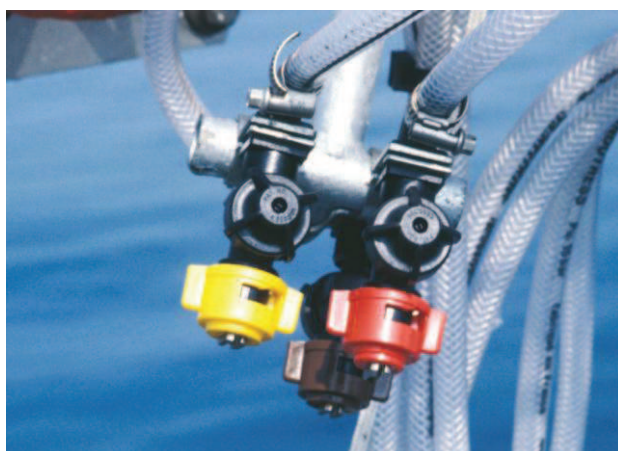
Nozzles fitted with check valves.
