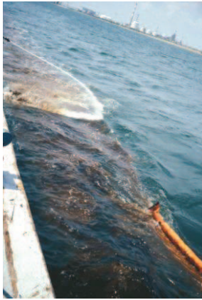
1., 2. Dispersion trial. See the beige colour of the slick just after spraying. This effect will last once a fire monitor has jetted the oil and dispersant.
