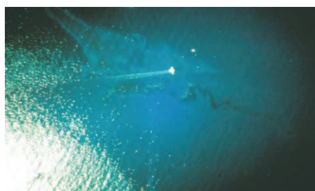
11. Continuation of treatment. Note the appearance of a dispersion cloud (beige yellow) upwind of the thicker patches (black) and also below, temporary disappearance of thinner patches (the herder effect a dispersant can produce but this is not real dispersion in action at all).
