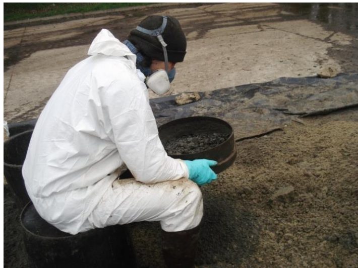
Manual sand sieving (Source: Le Floch Depollution)
