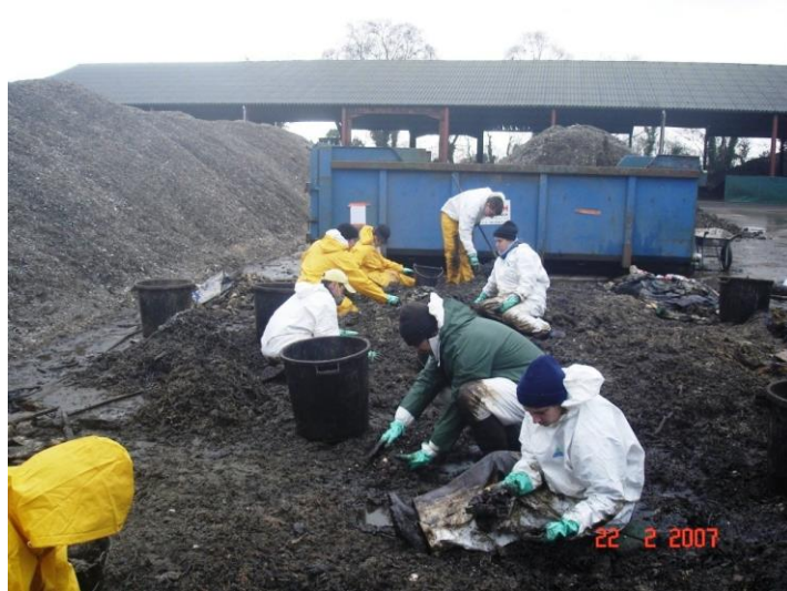
Sorting of waste prior to pre-treatment (required in the absence of sorting during collection) (Source: Le Floch Depollution)
