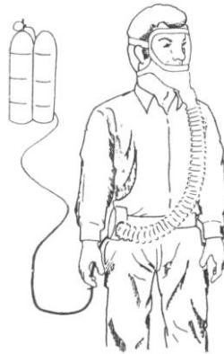
Figure 13: Air-line respirator arrangement
