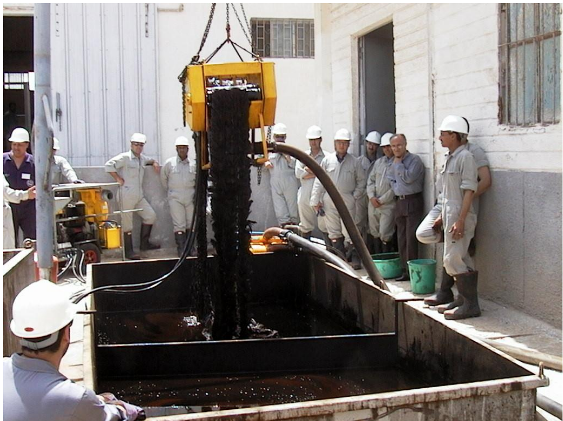
Demonstration of oil-mop skimmer
