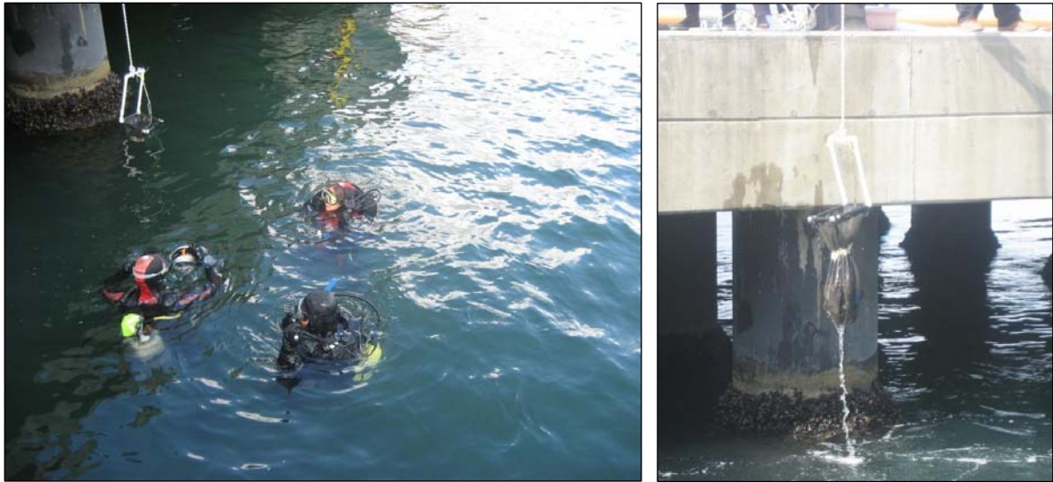
Fig. 5 & 6 - Collection of samples through pile scraping by means of divers. Samples collected underwater were put in a collection bag attached to the quadrat which was retrieved from the surface.
