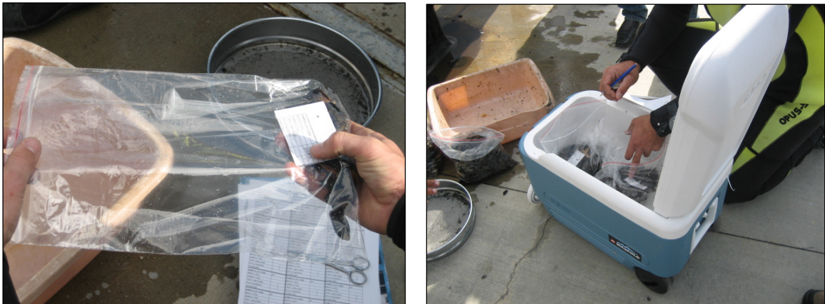
Fig. 9 & 10 – The samples collected were labeled and kept refrigerated in a sample cooling box until their arrival in the laboratory.
