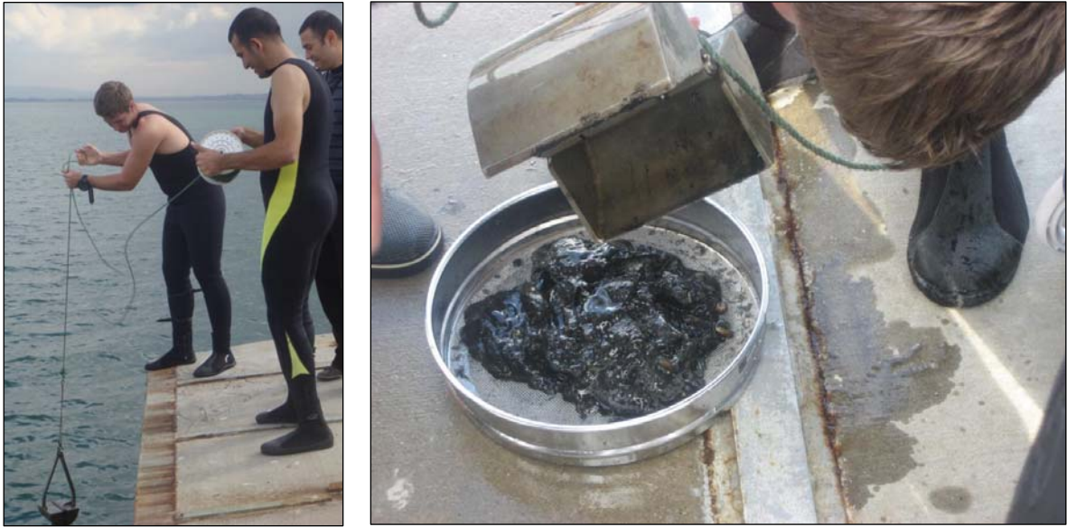
Fig. 7 & 8 – Collection of samples through a Schipeck sediment grab.
